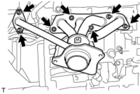
13. REMOVE NO. 2 EXHAUST MANIFOLD HEAT INSULATOR
