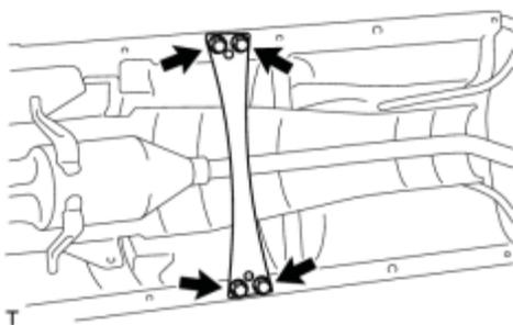
(a) Install the front center floor brace with the 4 bolts.
