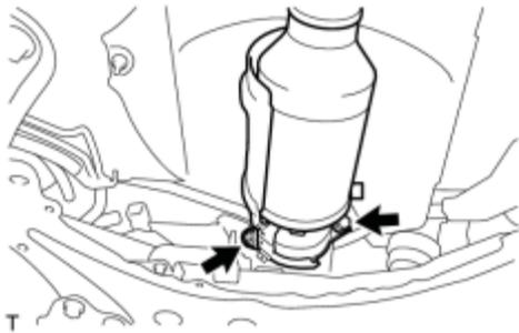
(b) Remove the 2 bolts and 2 compression springs.
