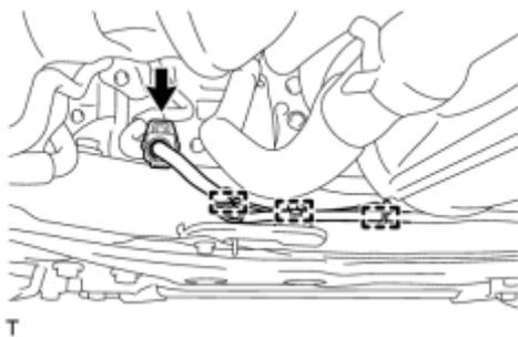
8. INSTALL FRONT EXHAUST PIPE ASSEMBLY (w/o Exhaust Heat Recirculation System)
