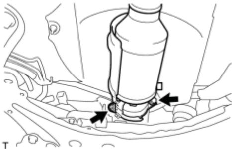
(e) Install the front exhaust pipe assembly with the 2 bolts and 2 compression springs.
