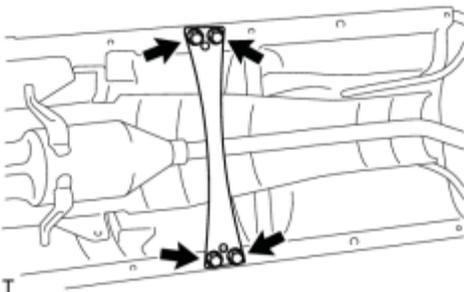
(a) Remove the 4 bolts and front center floor brace.
