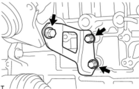
(a) Install the manifold stay with the 3 bolts.
