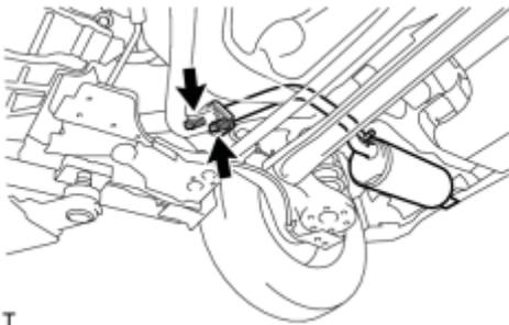
(e) Install the tail exhaust pipe assembly with the 2 bolts and 2 compression springs.
