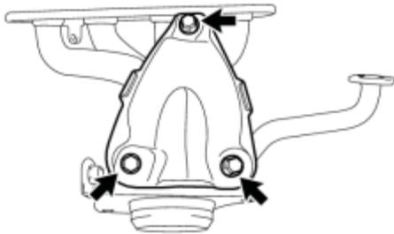
(a) Remove the 3 bolts and No. 2 exhaust manifold heat insulator.
