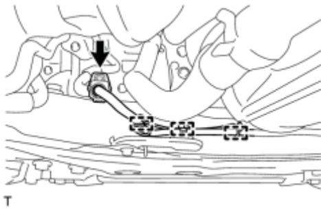
(a) Disconnect the 3 clamps and oxygen sensor connector.
