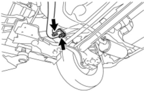
(e) Install the front exhaust pipe assembly with the 4 bolts and 4 compression springs.
