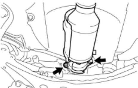
(a) Remove the 4 bolts and 4 compression springs.
