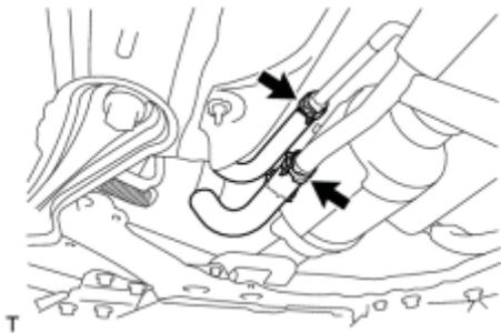
(b) Disconnect the 2 heater water hoses.
