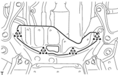
(a) Remove the 4 clips and front No. 3 engine under cover.
