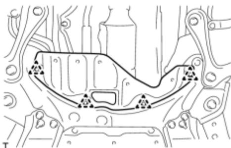
(a) Install the front No. 3 engine under cover with the 4 clips.
