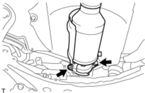
(a) Remove the 2 bolts and 2 compression springs.
