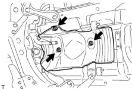
(a) Install the No. 1 floor heat insulator with the 3 nuts.
