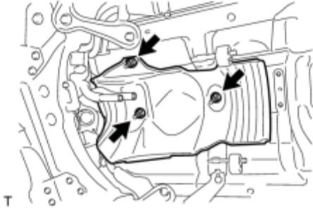
(a) Remove the 3 nuts and No. 1 floor heat insulator.
