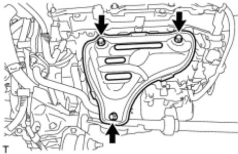
(a) Remove the 3 bolts and No. 1 exhaust manifold heat insulator.
