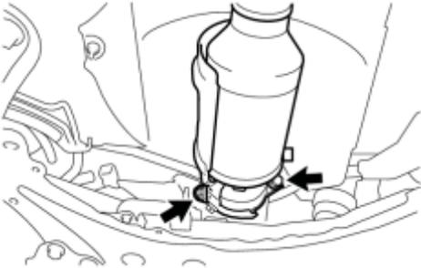
(d) Remove the front exhaust pipe assembly from the 3 exhaust pipe supports.
