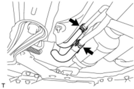
(a) Disconnect the 2 heater water hoses.
