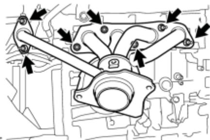
(a) Install 2 new gaskets and the exhaust manifold with the 7 nuts.
