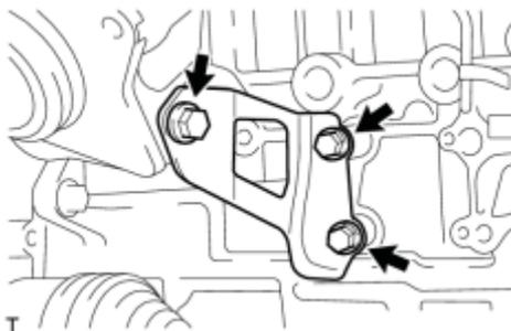
(a) Remove the 3 bolts and manifold stay.
